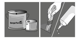
3. If using Stamcoll N55 Glue to fix the material, shake the tin thoroughly and fill the supplied applicator bottle to apply the glue to the substrate (wood, aluminium, steel, concrete, etc). Use a brush to spread the glue in 50 mm wide strips, three strips per full width of Stamisol Safe One (e.g. each side and middle). Coverage guide: 40 g of Stamcoll N55 per lin.meter.
